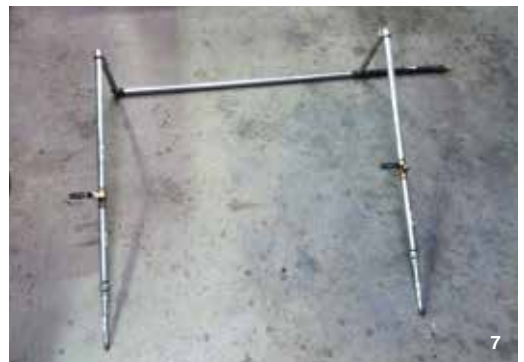
1 Wood-soda kiln with distribution manifold installed. 2 Gravity feed system into distribution manifold. 3 Close-up of WVO feeding into the kiln. 4 Burners being used. 5 Burner form with foam trough insert. 6 Finished castable burners. 7 Distribution manifold for wood-soda kiln.
