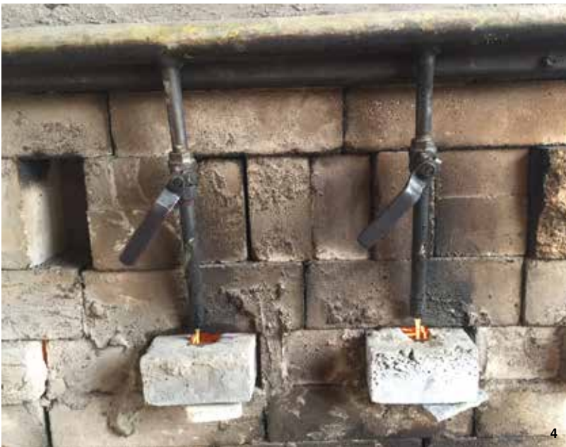
1 Wood-soda kiln with distribution manifold installed. 2 Gravity feed system into distribution manifold. 3 Close-up of WVO feeding into the kiln. 4 Burners being used. 5 Burner form with foam trough insert. 6 Finished castable burners. 7 Distribution manifold for wood-soda kiln.
